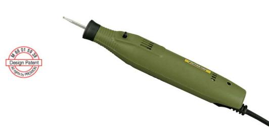
The engraver GG 12 spins at 20,000 rpm, yet weighs only 4 ounces! It allows for easy control and thus very safe operation featuring a touch sensitive switch for easy use and a simple push in/pull out shaft holder for easy accessory changeover (shaft capacity Ø 3/32" (2.35mm) only). The unit comes with 1 diamond bit with spherical head size 5/64" (1.8mm). Engrave for hours without fatigue.
